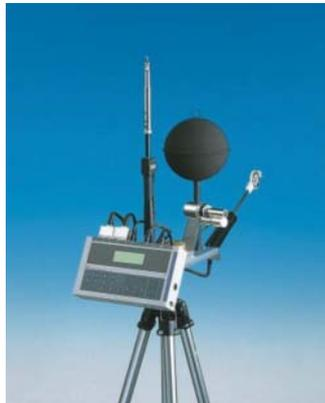
Fig. 1: The data acquisition System BABUC and two examples of microclimatic measurement (winter and summer – Indépendance square)
